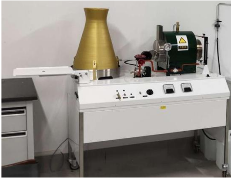
Fig. 3 Rankine Cycle Experimental System
